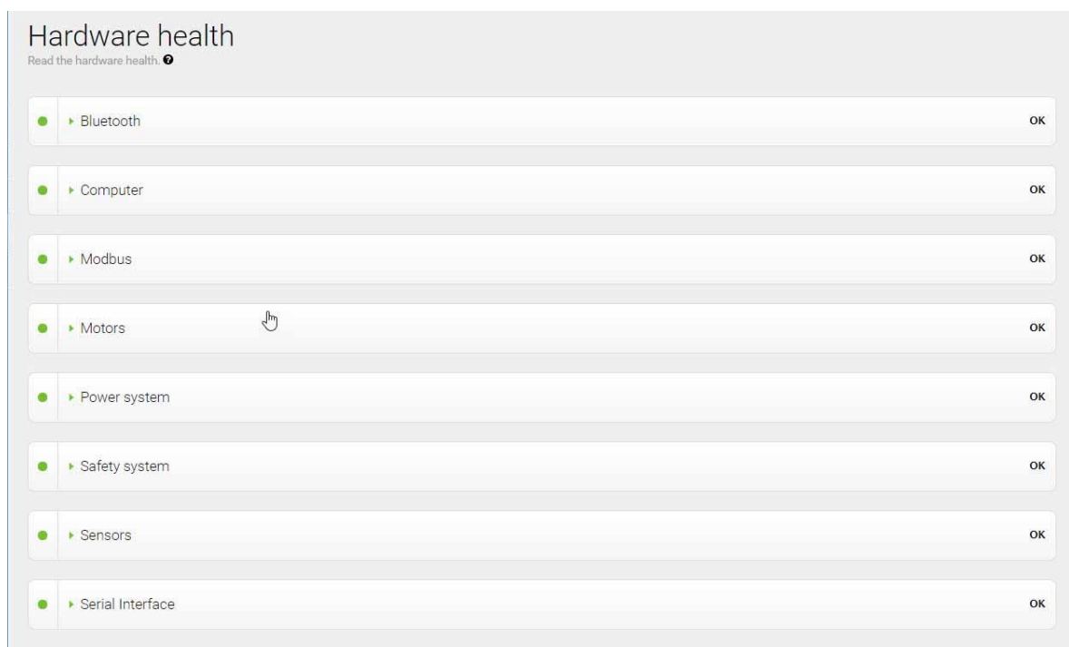
Figure 16.1. The interface in Hardware health displays which component is failing and often for what reason.
