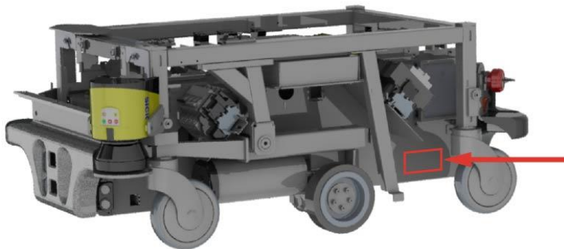
Figure 2.2. Placement of the identification label.
