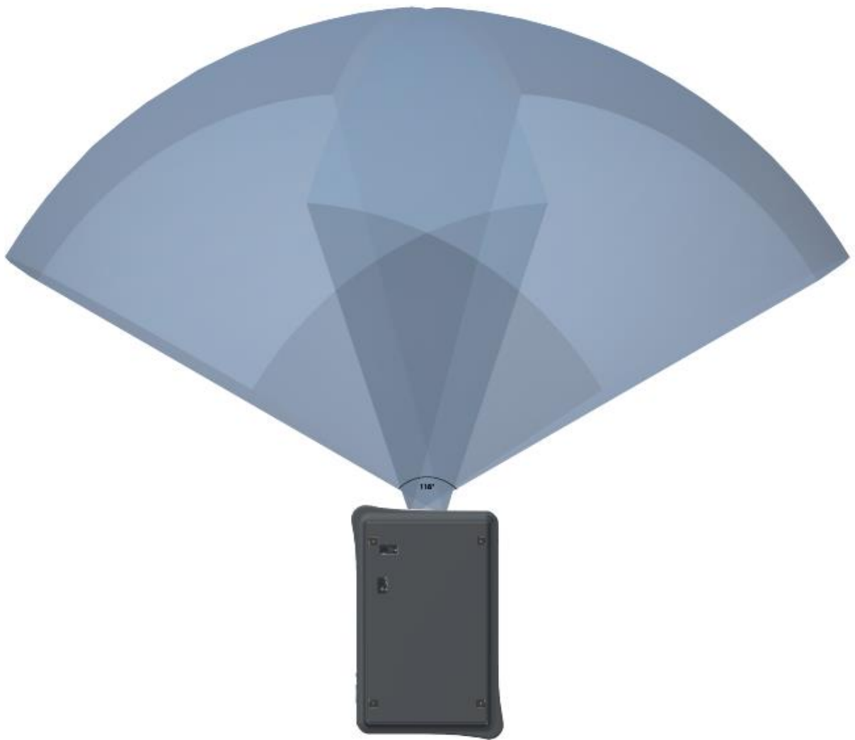
Figure 7.9. The two 3D cameras have a horizontal view of 118°.
