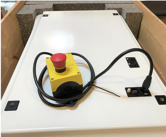
Figure 8.1. MiR100 has one Emergency stop button that must be connected through the electrical interface. You can also connect the interface to a series of additional Emergency stop buttons.
